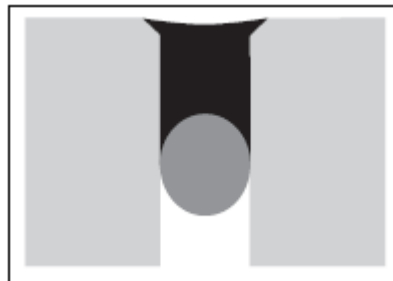
The flush joint design rules out trip hazards and dirt traps.
