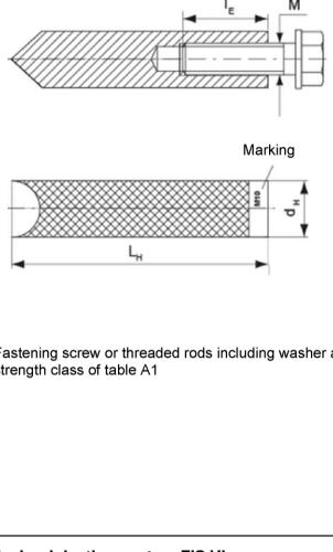
Marking: anchor size e.g.: M10 Stainless steel in addition A4 e.g.: M10 A4 High corrosion-resistant steel in addition C e.g.: M10 C
