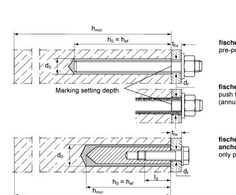
fischer threaded rod pre-positioned anchorage
